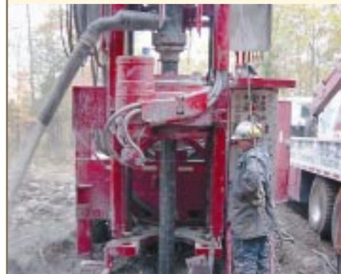
DR-24 shown in typical domestic waterwell application. Note the discharge swivel atop the casing which diverts the cuttings.
