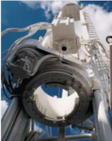
Lower drive feeds on two directly connected hydraulic cylinders (outside left & right). The top-drive feeds on a separate cylinder (center).
