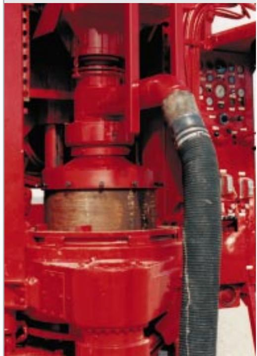
Standard discharge swivel sizes are 10" (254 mm), 16" (406 mm) and 24" (610 mm) and can accommodate 3 1/2" (89 mm) to 18" (457 mm) diameter drill pipe. Discharge swivel adapters allow the swivel to be fitted to other casing sizes.
