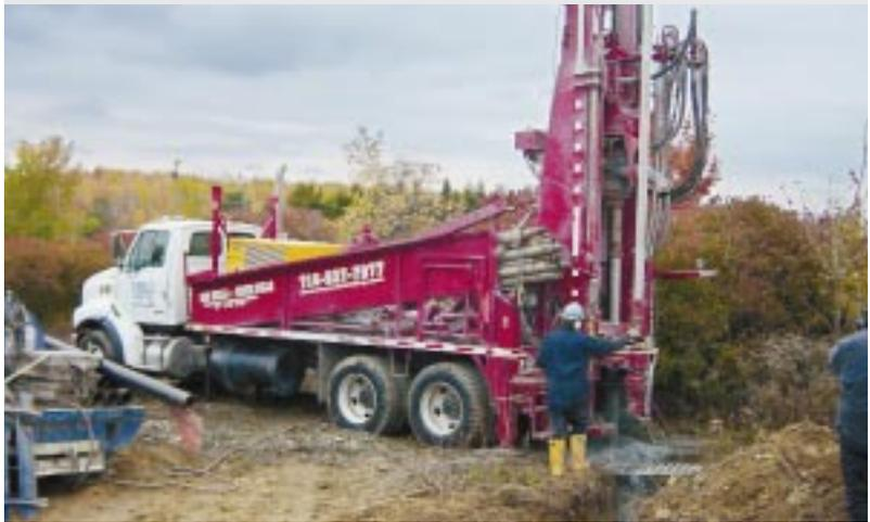
DR-12 with optional pipe tub and single rod loader in domestic waterwell application
